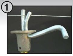
Place one Klaw Klip into the socket of the Application Tool and place wire between Klaws.
